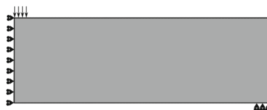
Fig. 25 Design space of 3 \times 1 and boundary conditions of the topology optimization problem. The vertical displacement is constrained at the right bottom, and a vertical load is applied at the left top. The horizontal displacement is constrained at the left boundary, which imposes a symmetry condition, such that the problem setup resembles a simply supported beam
