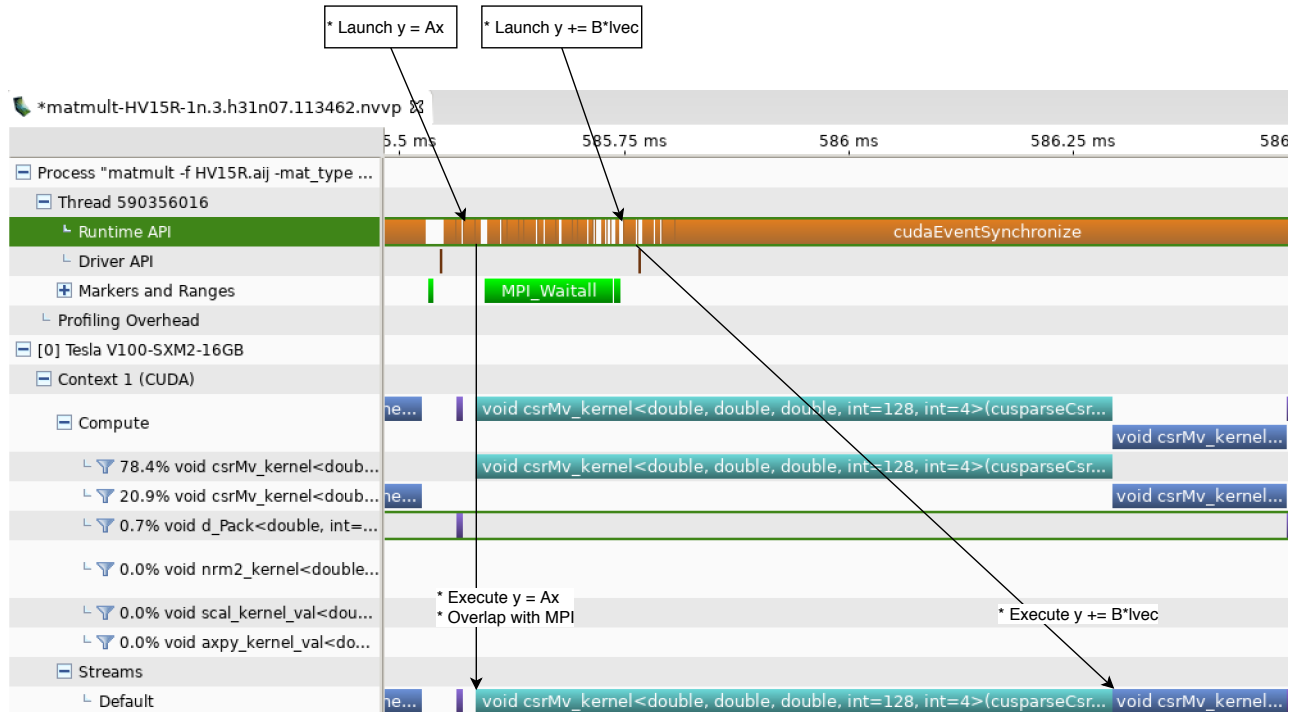
Figure 13: Timeline of MatMult with early launch of y = Ax . Note launch of kernel y = Ax does not need to wait for finish of the Pack kernel, but kernel y += B*1vec can not start until kernel y = Ax is completed.
