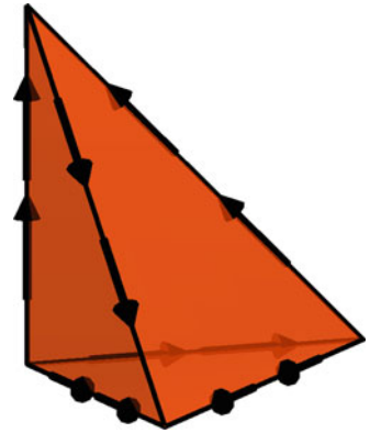
Figure 3.11: Illustration of first, second and third degree Nédélec H(\text{curl}) elements of the second kind on triangles. Note that these elements may be viewed as rotated Brezzi–Douglas–Marini elements.
