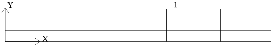
Figure 1: 5 \times 3 mesh generated by genbox .
