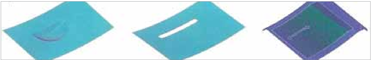
Fig. 4: Left image - FE model of contact surface of stamping die. Center image: FE model of flat panel geometry. Right image - Model of tool & material combined
